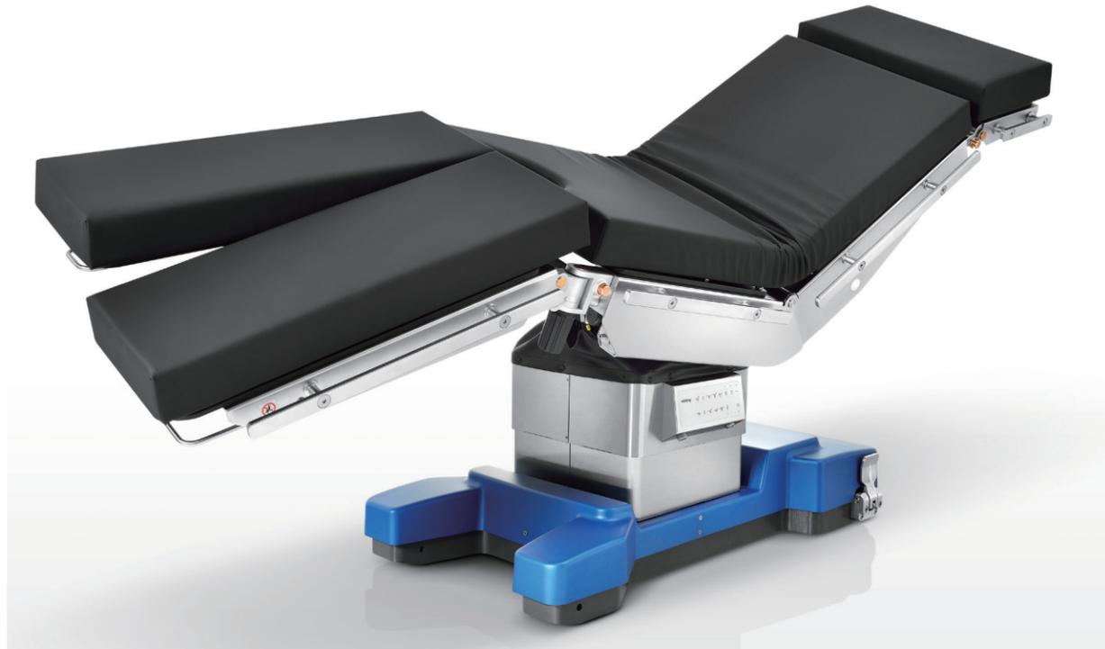
Providing a better clinical use's scenario, HyBase 6100 is designed with a much lower table height of 498mm specially for neurosurgery and minimally invasive surgery, a more user friendly base cover, as well as a more convenient wireless remote control system. Moreover, with longitudinal slide up to 320 mm, the table is ideally suitable for cardiovascular surgery or spinal surgery with C-arm. All in all, HyBase 6100 maximizes the flexibility of operating table's versatility.
